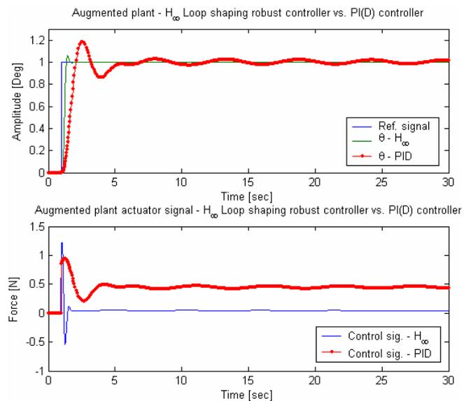
**Fig.11** Comparison of  $H_\infty$  Loop Shaping vs. PI(D).
