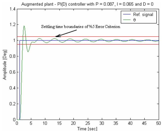
Fig.4 Time domain response of PID control system.
