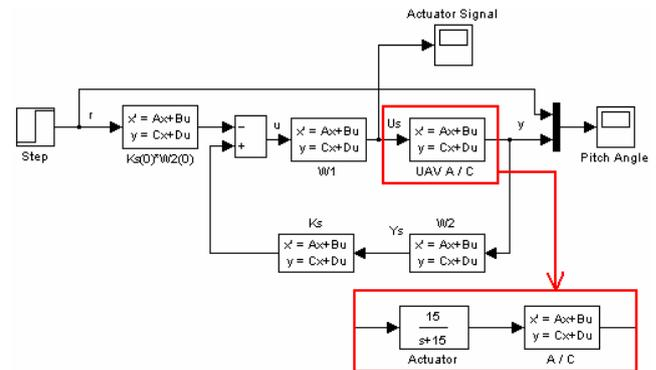
Fig.7  $H_\infty$  Loop Shaping control system block diagram.
