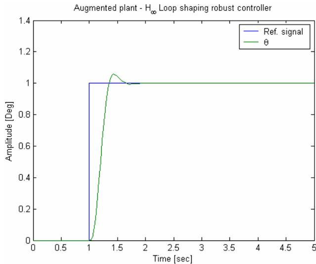
**Fig.8** Closed loop time domain response of  $H_\infty$  Loop Shaping robust control system.
