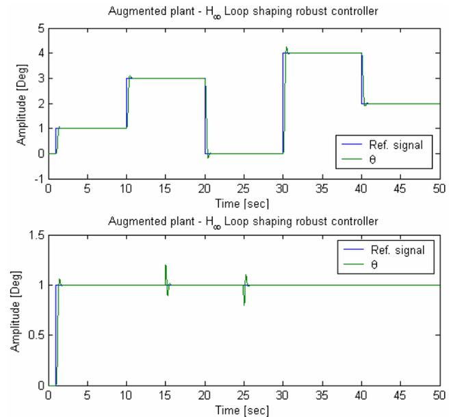
**Fig.10** Tracking and disturbance rejection of  $H_\infty$  Loop Shaping controller, respectively.
