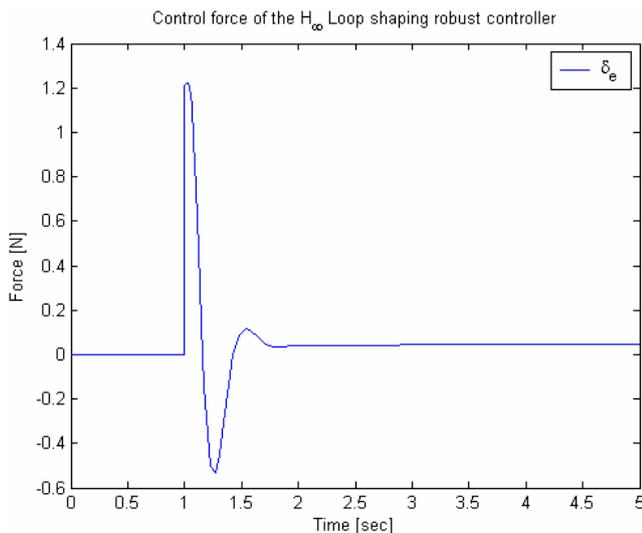
**Fig.9** Control force imposed by the actuator on the nominal plant.
