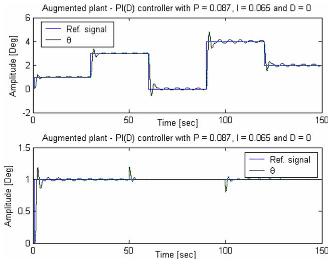
Fig.6 Tracking and disturbance rejection of PI(D) controller, respectively.
