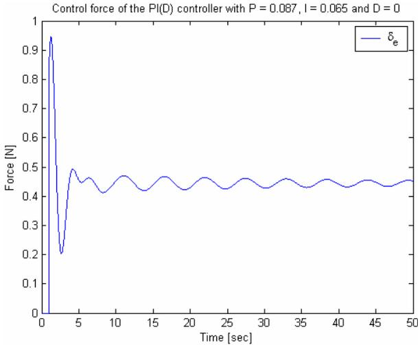
Fig.5 Control signal imposed by the actuator.
