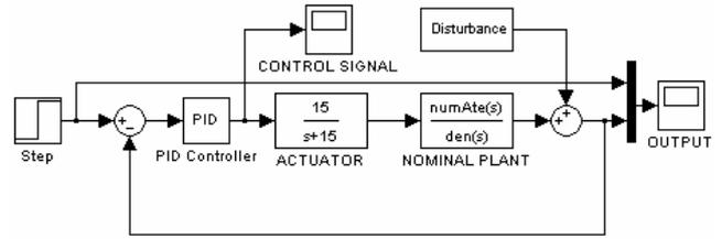
Fig.3 PID flight control system block diagram.
