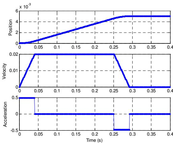
Fig. 2. Typical set of simulated reference inputs based on trapezoidal velocity profile.
