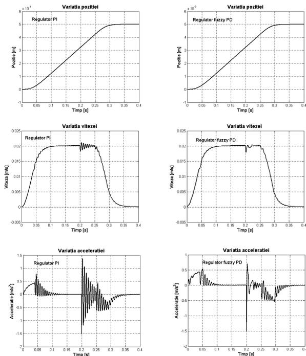
Fig. 4. Comparison between digital PI and fuzzy PD controllers
