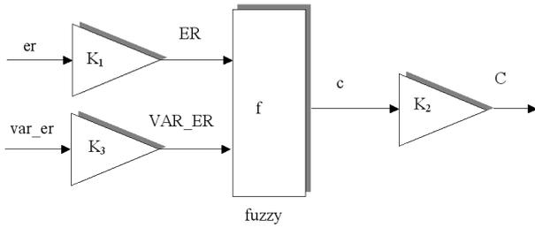
Fig. 3. The internal structure of the fuzzy controller
