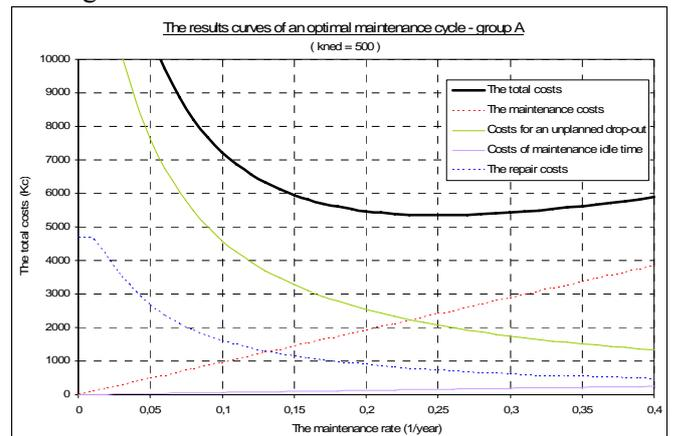
Fig. 2 The curves necessary for the optimizing of maintenance cycle - e.g. for group A,  $k_{ned} = 500$
