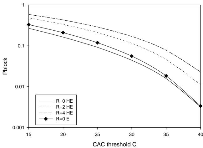
Figure 4: New call blocking prob. vs. CAC threshold and guard channels with NCAC
