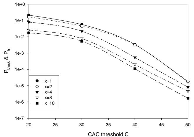
Figure 1: New call blocking and handoff failure prob. vs. CAC threshold and burstiness with NCAC
