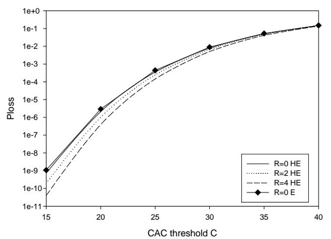
Figure 7: Packet loss probability vs. CAC threshold and guard channels with NCAC
