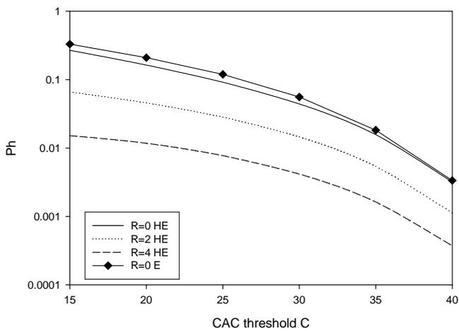
Figure 5: Handoff failure prob. vs. CAC threshold and guard channels with NCAC
