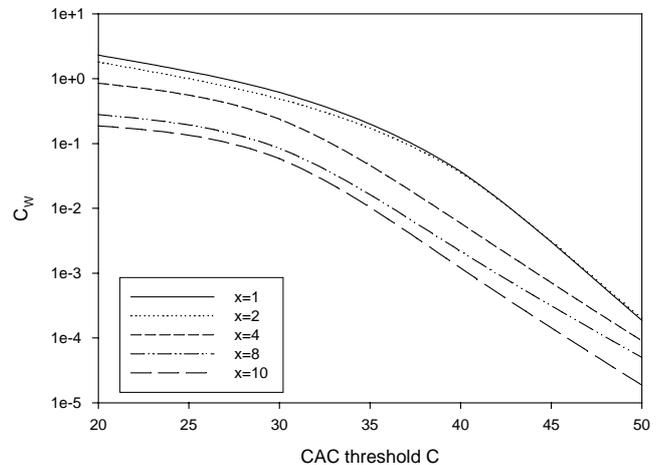
Figure 2: Weighted cost vs. CAC threshold and burstiness with NCAC
