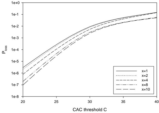
Figure 3: Packet loss prob. vs. CAC threshold and burstiness with NCAC
