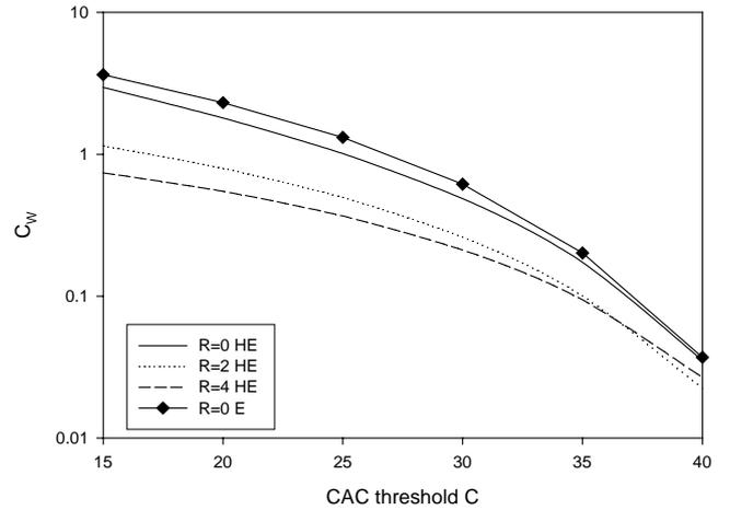
Figure 6: Weighted cost vs. CAC threshold and guard channels with NCAC
