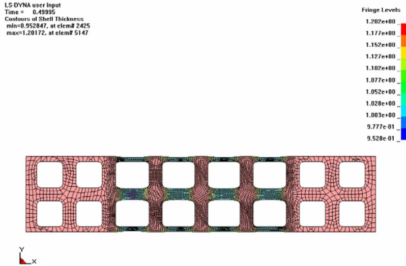
Fig. 8 Numerical results in the plate with square holes (D= 10 mm) placed in parallel
