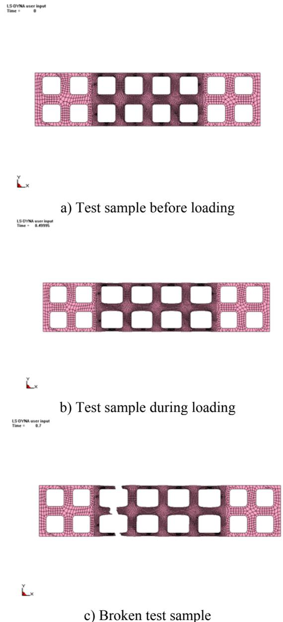
Fig. 6 Aspect of the test sample at various stages during the experiment
