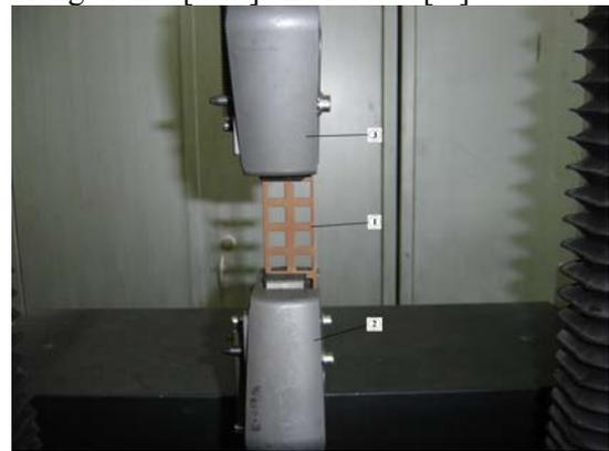
**Fig. 3** Test sample made of a perforated metal sheet with squared holes
