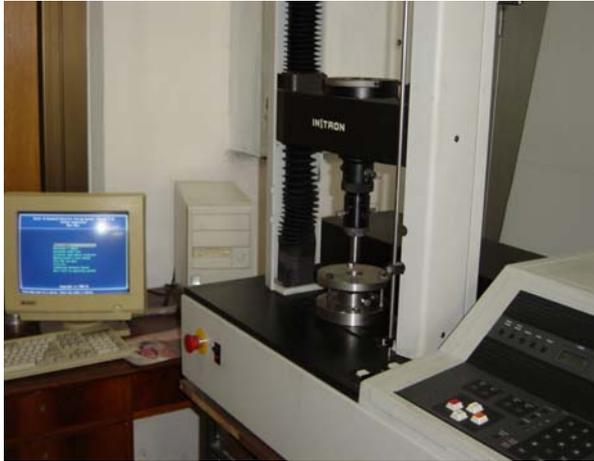
**Fig. 2** The universal traction, compression and buckling testing machine INSTRON 4303
