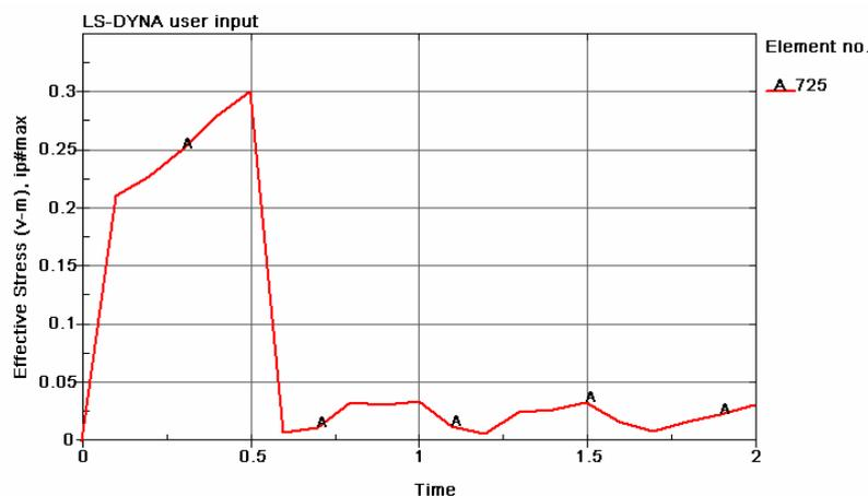
Fig. 7 Variation of the equivalent stress for an element
