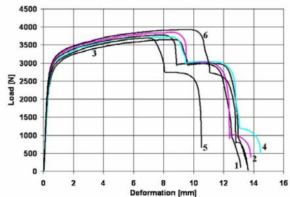
**Fig.4** Characteristic tensile stress-strain curves for a metal sheet of 0.8 [mm] thickness with squared holes in parallel pattern, stressed uniaxially.
