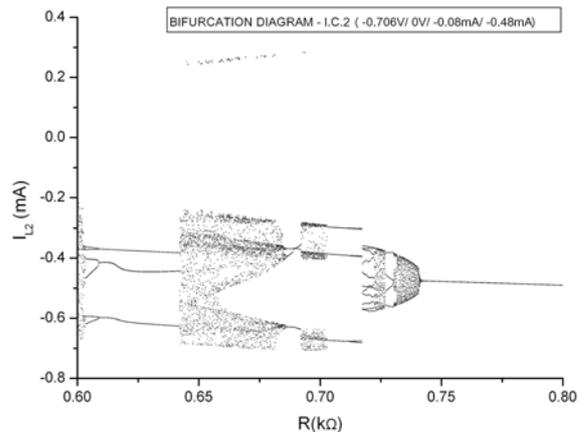
Fig.5. Bifurcation diagram  $i_{L2}$  vs.  $R_1$  for initial conditions 2 (i.c.2).
