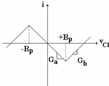
Fig.2. The v-i characteristic of nonlinear resistor RN.
