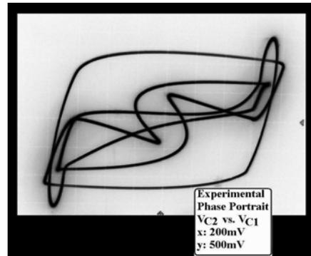
Fig.16. Experimental diagram  $v_{C2}$  vs.  $v_{C1}$  (period-3).
