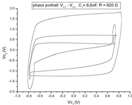
Fig.12. Phase portrait  $v_{C2}$  vs.  $v_{C1}$  for  $R_1=620.0\Omega$  ( $LE_1=0, LE_2=-0.069<0, LE_3=-0.079<0$ --period-3).
