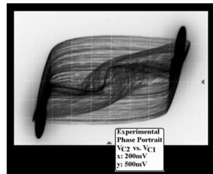
Fig.17. Experimental diagram  $v_{C2}$  vs.  $v_{C1}$  (chaos).
