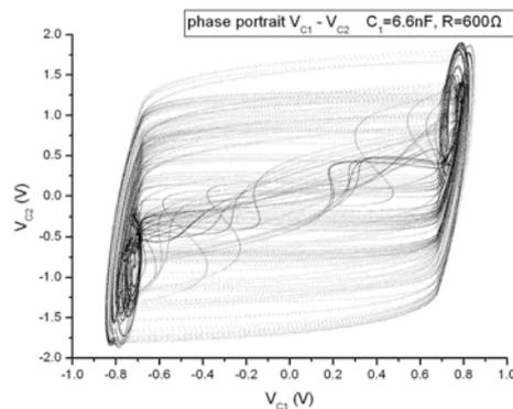
Fig.9. Phase portrait  $v_{C2}$  vs.  $v_{C1}$  for  $R_1=600.0\Omega$  ( $LE1=0.034>0, LE2=0, LE3=-0.10<0$ --chaos).
