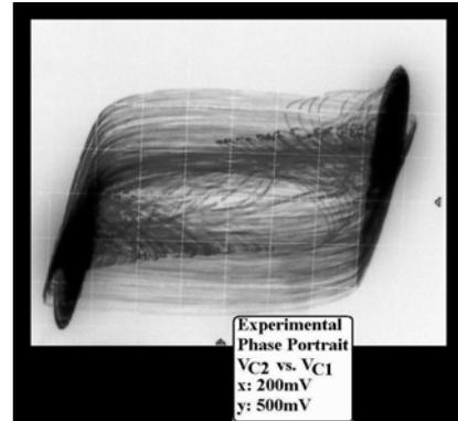
Fig.14. Experimental diagram  $v_{C2}$  vs.  $v_{C1}$  (chaos).
