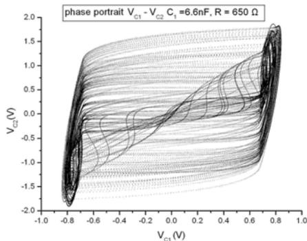
Fig.13. Phase portrait  $v_{C2}$  vs.  $v_{C1}$  for  $R_1=650.0\Omega$  ( $LE_1=0.0466>0, LE_2=0, LE_3=-0.112<0$ --chaos).
