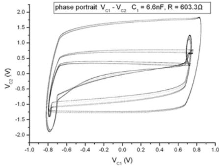
Fig.10. Phase portrait  $v_{C2}$  vs.  $v_{C1}$  for  $R_1=603.3\Omega$  ( $LE_1=0, LE_2=-0.031<0, LE_3=-0.121<0$ --period-12).
