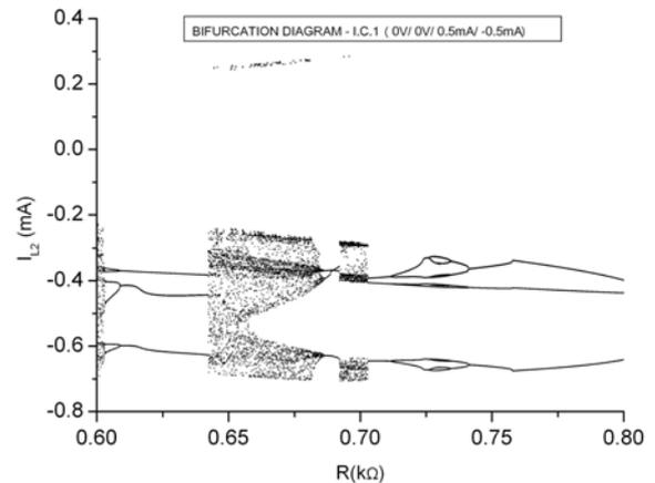
Fig.4. Bifurcation diagram  $i_{L2}$  vs.  $R_1$  for initial conditions 1 (i.c.1).
