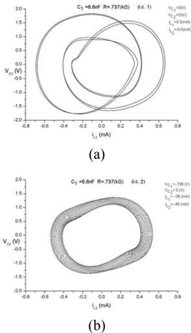
Fig.7. Phase portrait  $v_{C2}$  vs.  $i_{L2}$  for  $R_1=737\Omega$  and initial conditions (a) i.c.1--periodic ( $LE1=0, LE2<0, LE3<0, LE4<0$ ) (b) i.c.2--quasiperiodic ( $LE1=0, LE2=0, LE3<0, LE4<0$ ).
