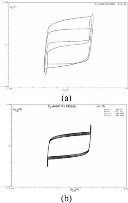
Fig.6. Phase portrait  $v_{C2}$  vs.  $v_{C1}$  for  $R_1=742\Omega$  and initial conditions (a) i.c.1--periodic ( $LE1=0, LE2<0, LE3<0, LE4<0$ ) (b) i.c.2--quasiperiodic ( $LE1=0, LE2=0, LE3<0, LE4<0$ ).
