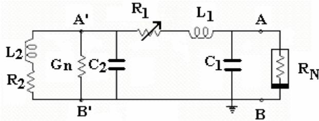
Fig.1. The fourth-order autonomous electric circuit.
