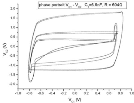
Fig.11. Phase portrait  $v_{C2}$  vs.  $v_{C1}$  for  $R_1=604.0\Omega$  ( $LE_1=0, LE_2=-0.0306<0, LE_3=-0.116<0$ --period-6).
