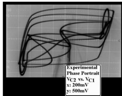
Fig.15. Experimental diagram  $v_{C2}$  vs.  $v_{C1}$  (period-6).
