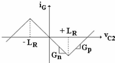
Fig.3. The v-i characteristic of negative conductance.
