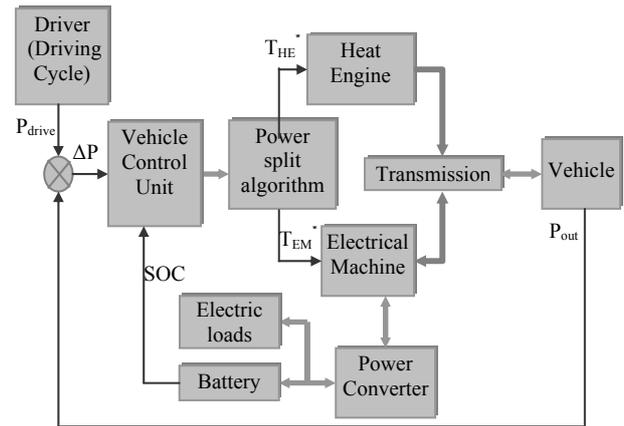
Fig.2. The model of a parallel HEV
