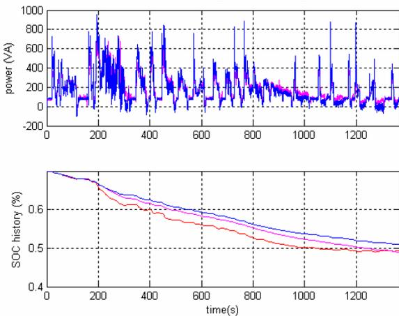
Fig.8. Time history of motor power and change in the battery storage energy
