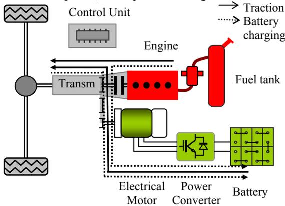
Fig.1. Parallel hybrid electric vehicle
