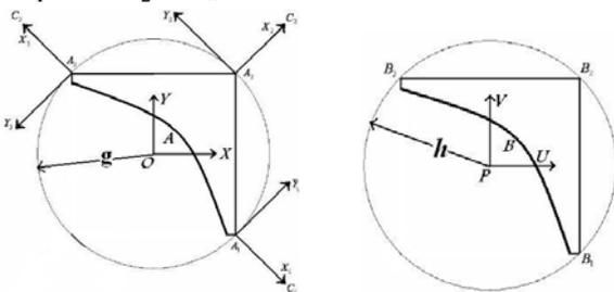
Fig. 2: Fixed and moving platforms
