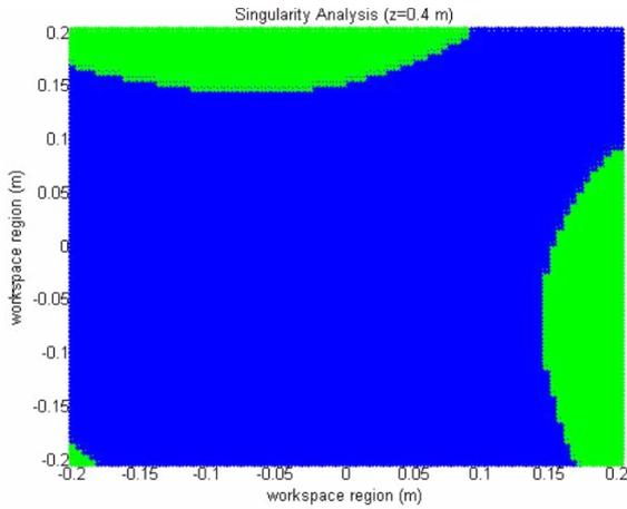
**Fig. 4:** Workspace singular points (critical plate)
