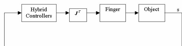
Fig.1 The slip control system
