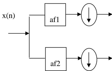
Fig. 1. Separable DWT (Analysis)
