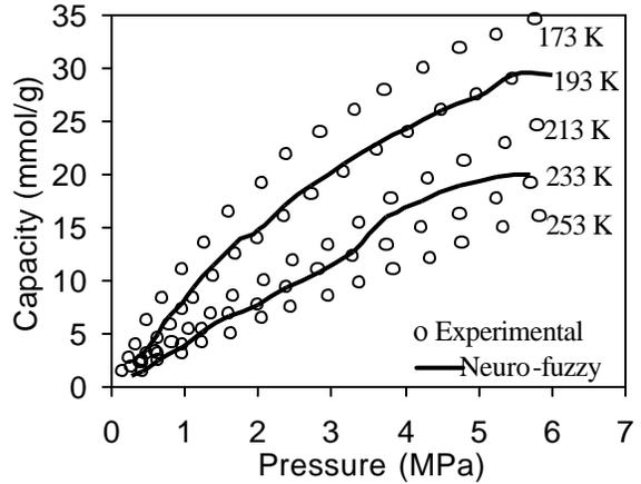
Figure 3: Model validation of hydrogen adsorption isotherm at temperature of 193 K and 233 K.
