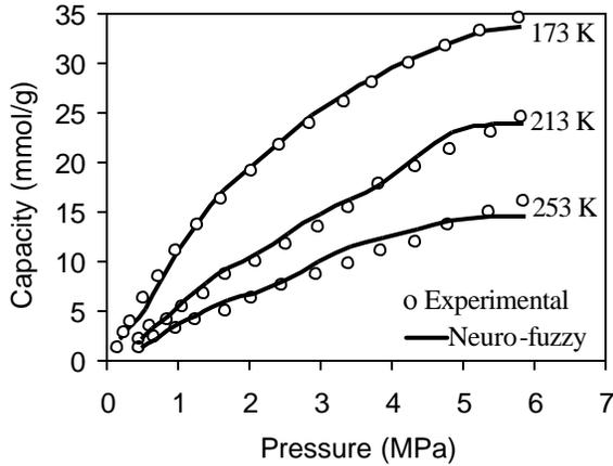
Figure 2: Comparison between isotherm model of hydrogen adsorption using Neuro-Fuzzy with experimental data (Zhan, 2004).
