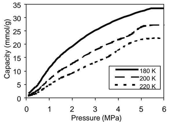
Figure 4: Prediction of hydrogen adsorption isotherm at various temperatures.
