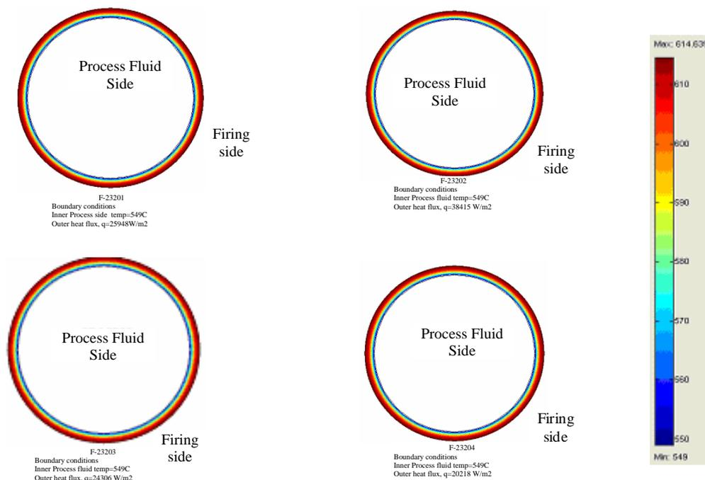
Fig. 11: The front view for tube skin temperature of Heater1: F-23201, Heater2: F-23202, Heater3: F23203, Heater4: F23204
