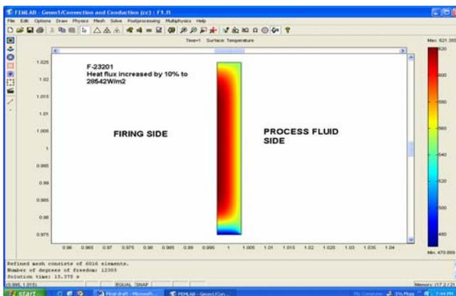
Fig 13: Effects of varying inlet and process fluid temperatures of Heater1.
