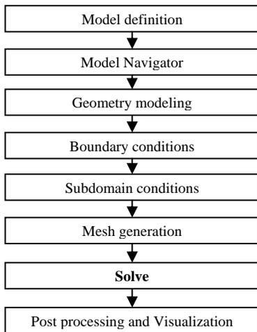
Fig.1: Flowchart in GUI of FEMLAB
