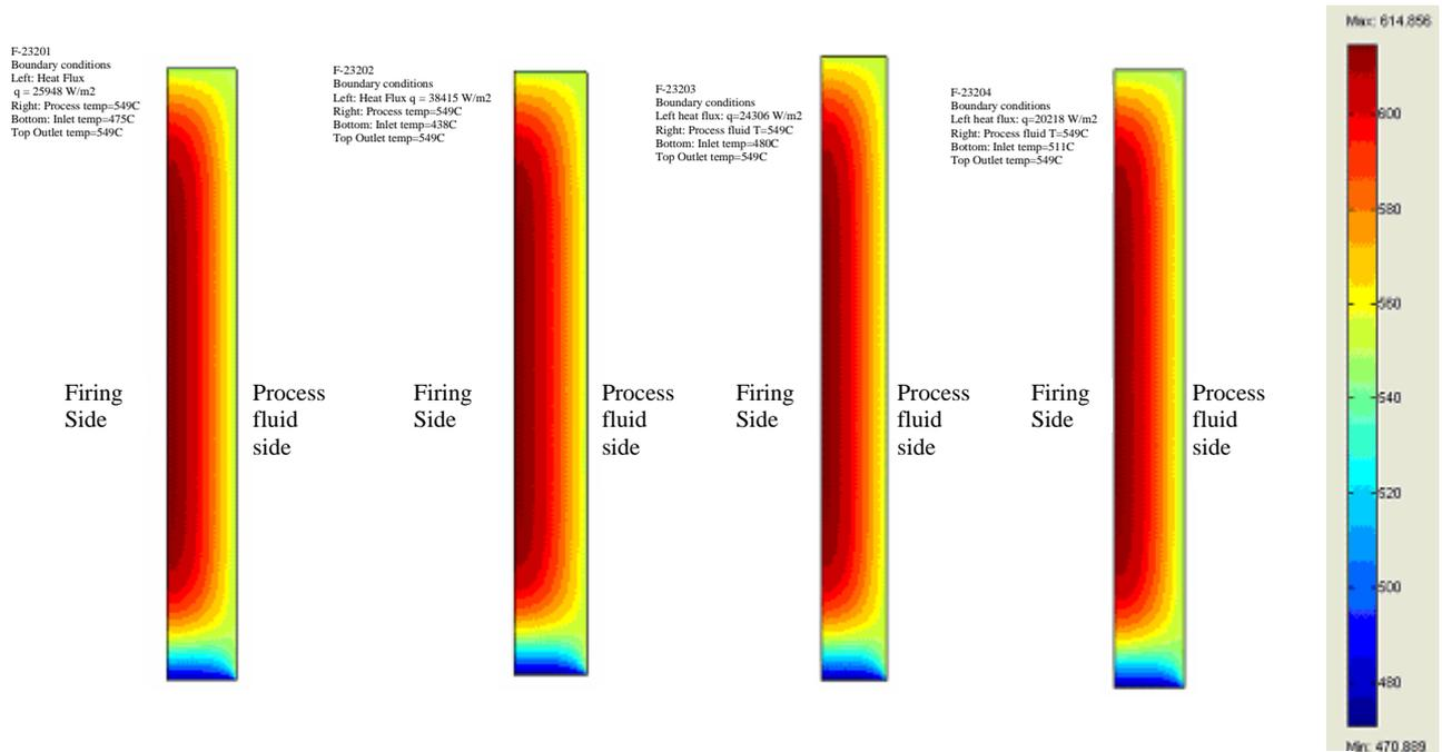
Fig. 10: The horizontal cross-sectional view for tube skin temperature of Heater1: F-23201, Heater2: F -23202, Heater3: F23203, Heater4: F23204
