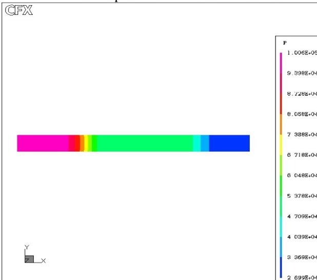
Fig.4 Pressure variations in shock tube, from the numerical results.
