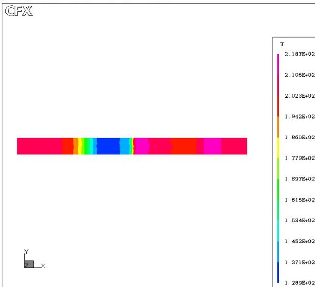
A contact surface follows the initial normal shock wave down the tube. This contact surface is a temperature discontinuity, separating the gases
