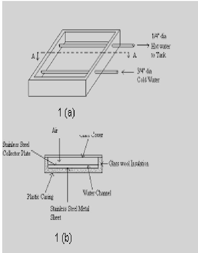
Figure 1 (a) Collector / Absorber Design, (b) X-Section AA
