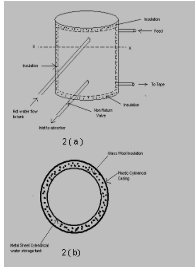
Figure 2 (a) Water Storage Tank, (b) Cross-section XX
