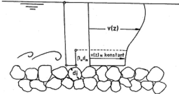
Fig. 4: Velocity profile for very rough flow
