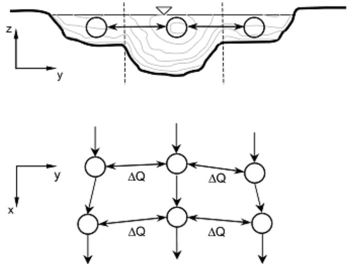
Fig.6: Concept of stream pipes for natural rivers with floodplains. The conservation of continuity, energy and momentum should be satisfied at every node. But a mass transfer is allowed in this model perpendicular to the flow direction [18].
