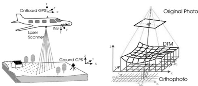
Fig.5: Principle of automatic grid generation with laser scanning [14]
