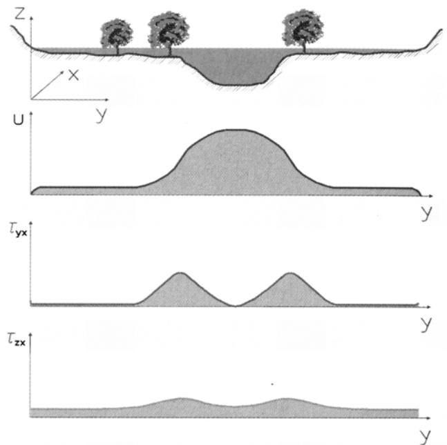
Fig.7: Idealized distribution of the velocity and shear stress in a natural river with floodplains. Measurements have to be done to verify and improve the used theory [10]
