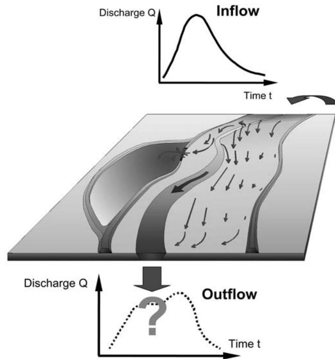
Fig. 1: Sketch of the deformation of a hydrograph in natural river flow with retention effects
