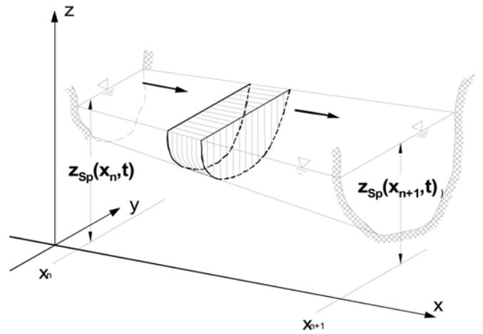
Fig. 2: Sketch of one dimensional flow
