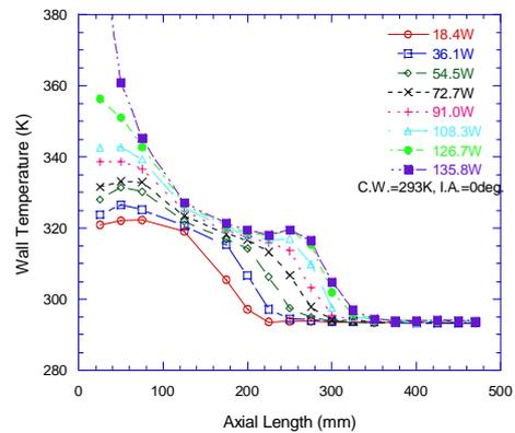
Fig.2. Wall temperature distribution with heat transport capacity (HP1)
