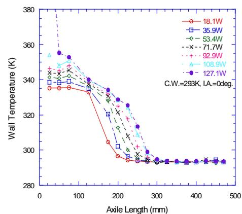
Fig.4. Wall temperature distribution with heat transport capacity (HP3)
