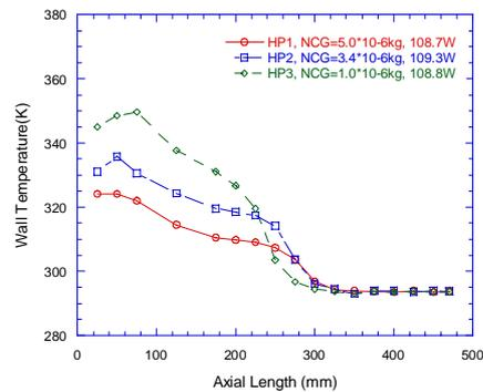
Fig.6. Wall temperature distribution with heat transport capacity at 110 W.
