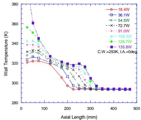
Fig.3. Wall temperature distribution with heat transport capacity (HP2)
