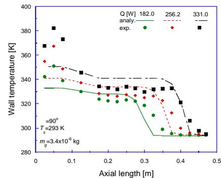
Fig.7. Comparison of the analyzed and experimental results for wall temperature with input power for HP2.
