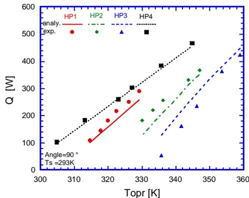
Fig.8. Comparison of the analyzed and experimental results for heat transfer rate with operating temperature in various heat pipes.
