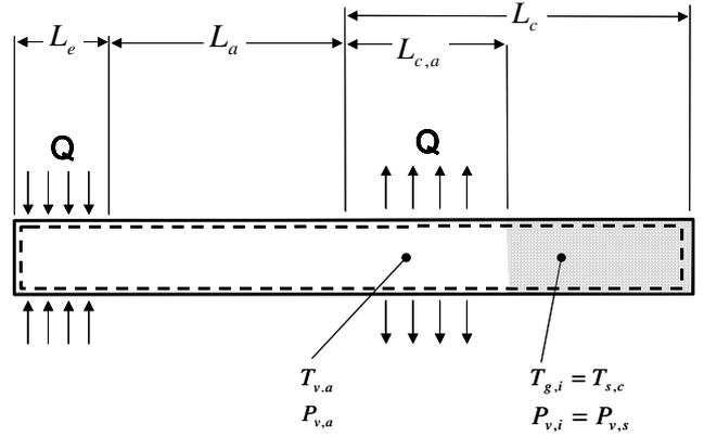
Fig.1. Schematic diagram of VCHP
