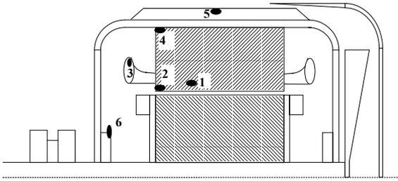
**Fig. 1 Axial view of the motor showing the locations of the sensors.**
