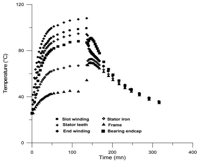
**Fig.5 Heating and cooling curves at full-load with ventilation**
