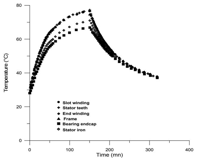
**Fig.4 Heating and cooling curves at no-load without ventilation**
