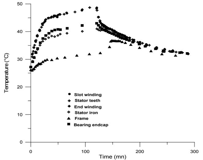
**Fig.3 Heating and cooling curves at no-load with ventilation**
