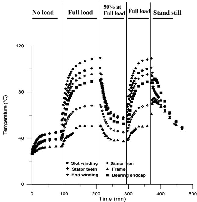
**Fig.6 Heating curves for several load conditions with ventilation**
