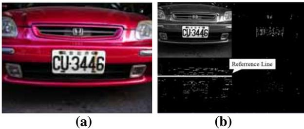
**Fig.2 (a) original input image (b) result of Haar wavelet transform and the reference line in LH subimage**
