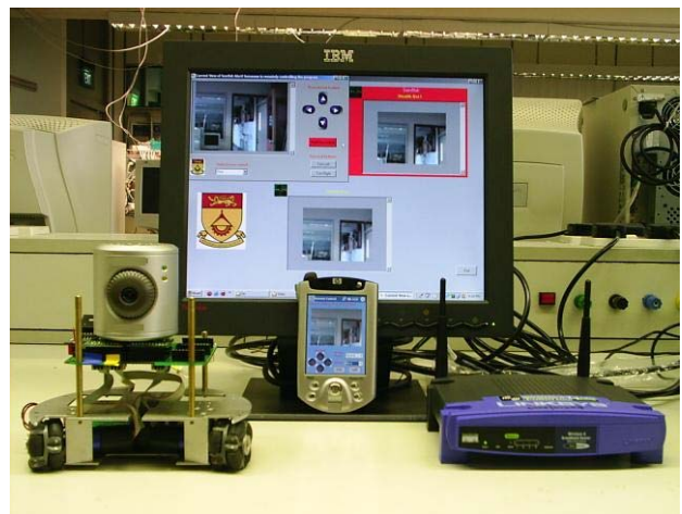
Fig.2 The mobile security system (security robot)
