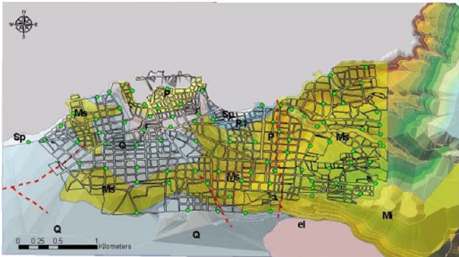
Figure 4. Map of the city of Chania. With green dots are the measurement points, colours indicate different geological formations.
