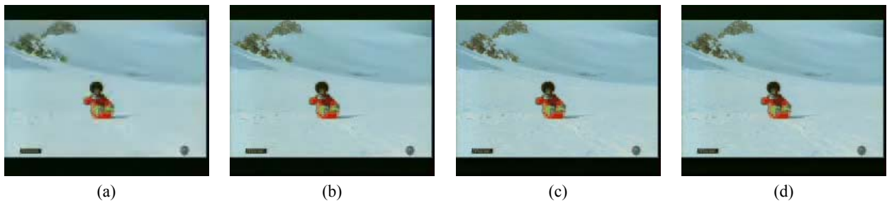
Fig. 4. Frames sampled from the marked video sequences, in the DCT domain. The video was coded at different bit rates: 64 kbit/s in (a), 128 kbit/s in (b), 192 kbit/s in (c), and 256 kbit/s in (d).
