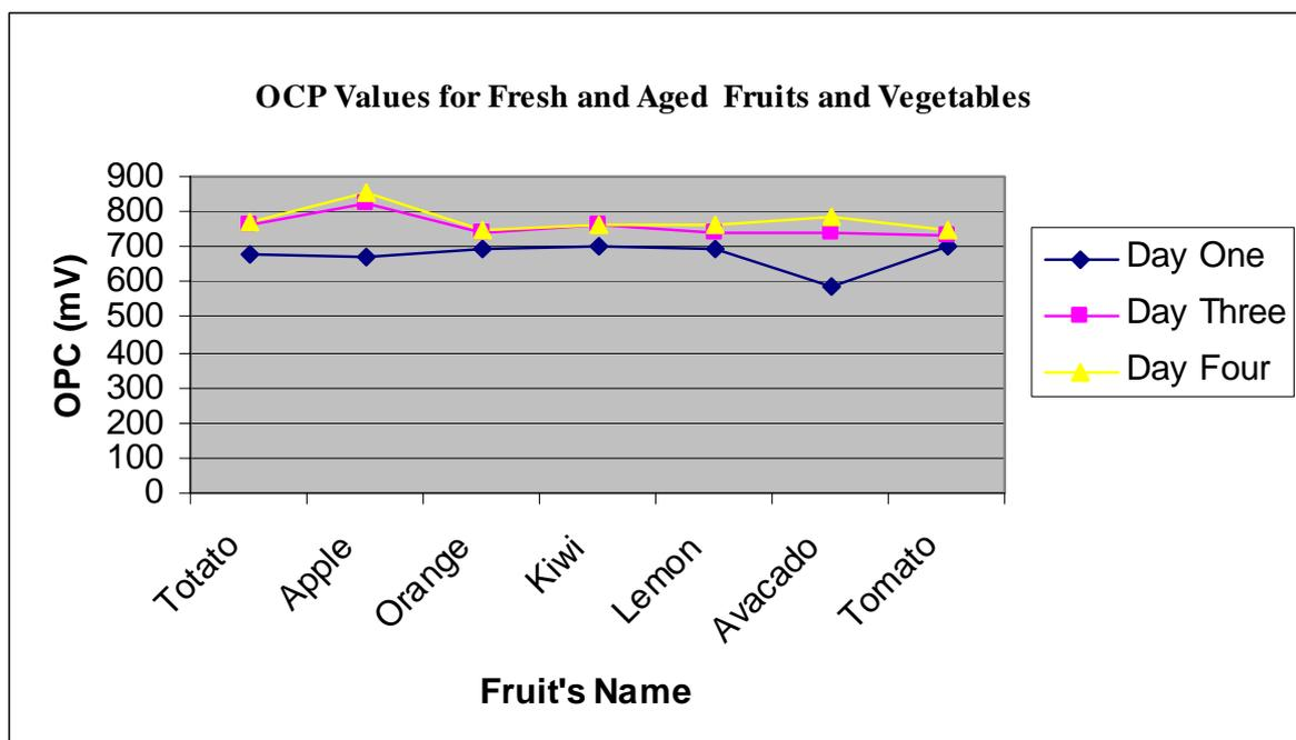
Figure-6: Aging-time Versus Voltage for Fruits and Vegetables
