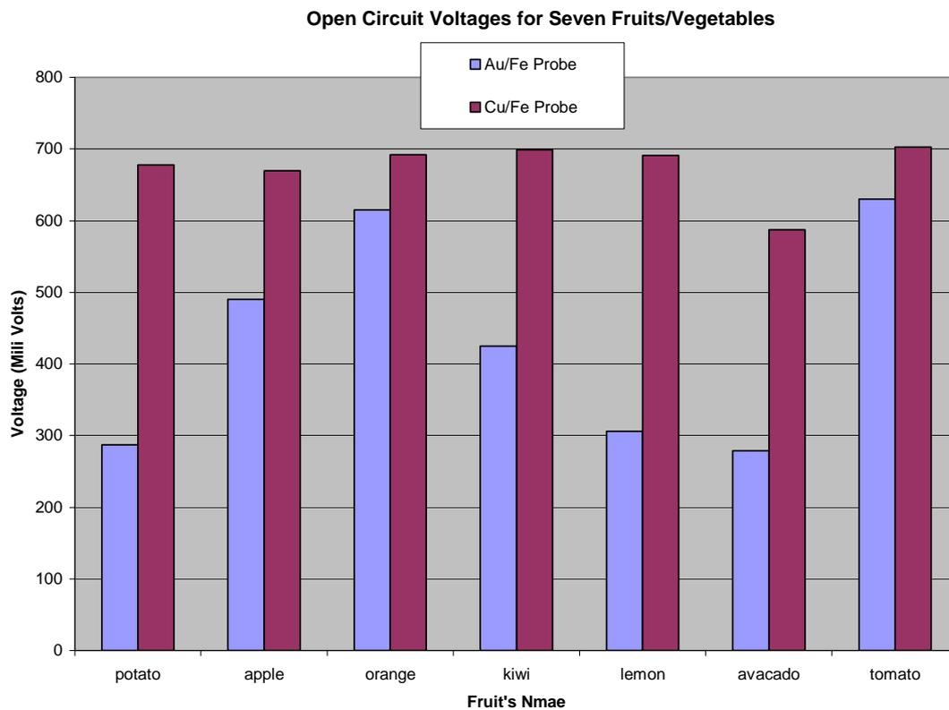
Figure-5: Column graph for seven fruits and vegetables using two different probes
