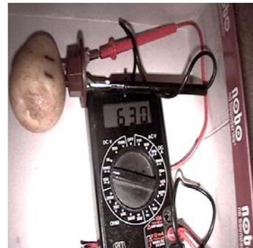
Figure 4: OCP Measurement in Progress
