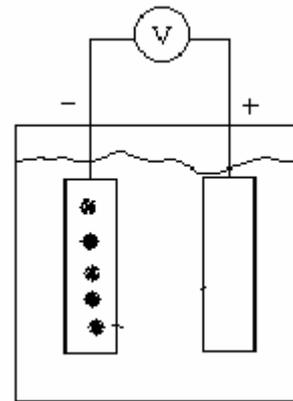
Figure-1. Configuration of a Wet Voltaic Cell
